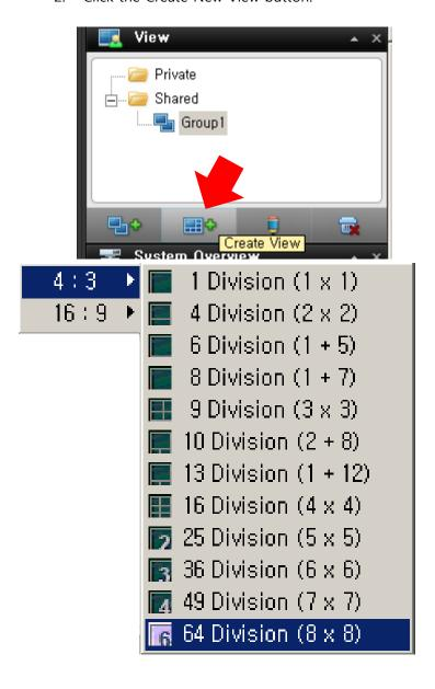
3. Select the required layout for your new view. You are able to select layouts for displaying up to 64 (8×8) cameras in a single view
