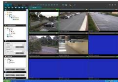
Tip: The SW supports use of multiple windows. This is especially useful if your computer has more than one physical display attached.
